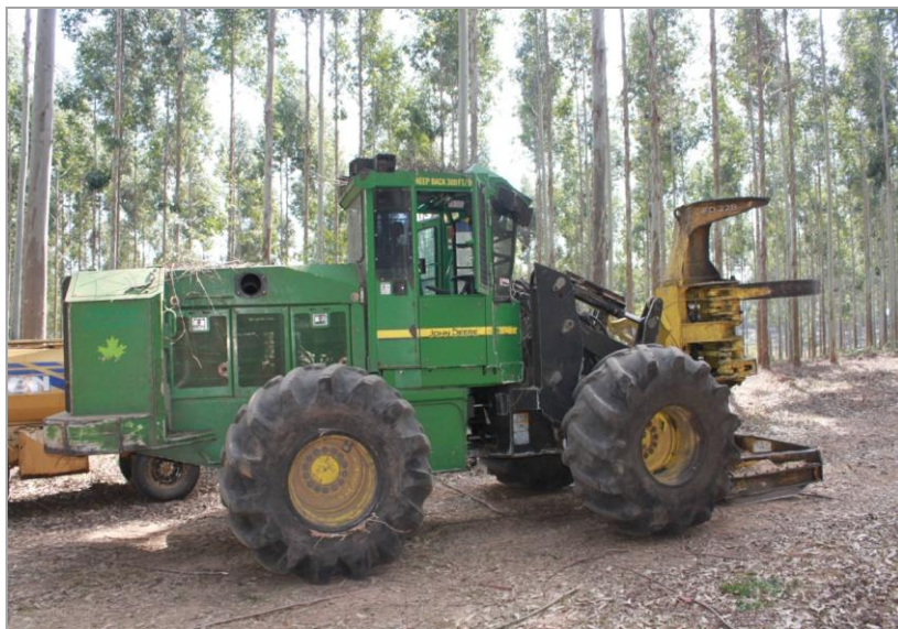
Figura No.6 Feller Buncher John Deere 843 k con cabezal FD 22B
