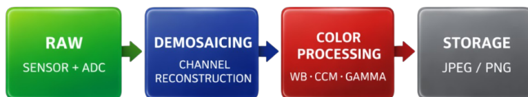
Figure 2.1: Simplified camera pipeline showing the main stages from sensor acquisition to compressed image storage.
