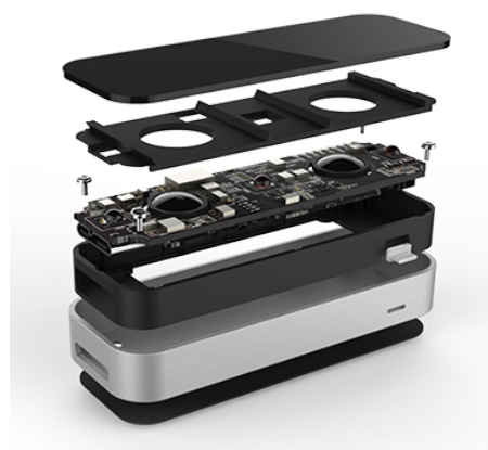
Figura 6: Componentes hardware del sensor Leap Motion [41]
