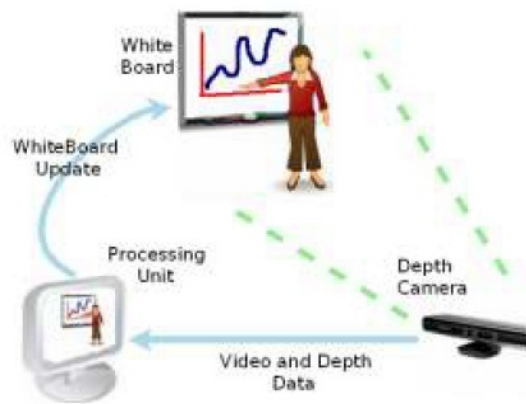
Figura 37: Arquitectura de sistema Low-Cost Efficient Interactive Whiteboard [75]
