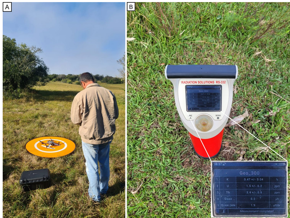
Fig. 3 (A) Drone DJI MAVIC 3 T; (B) RS-332 with results on the screen after measurement on Point 44
