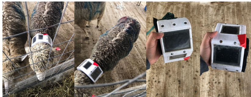
Figure 6.5: Post rain test confirming OVIS device resistance.
