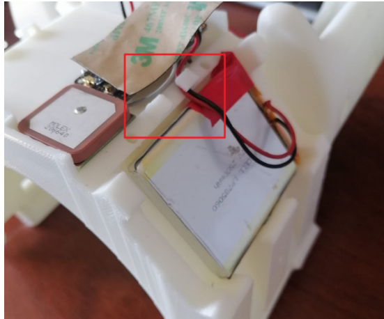
Figure C.3: Component placing inside OVIS device enclosure.
