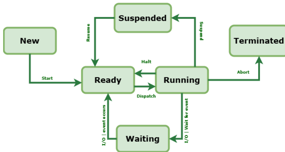
Figure 3.2: Thread state machine for Zephyr RTOS. Diagram inspired from [51].
