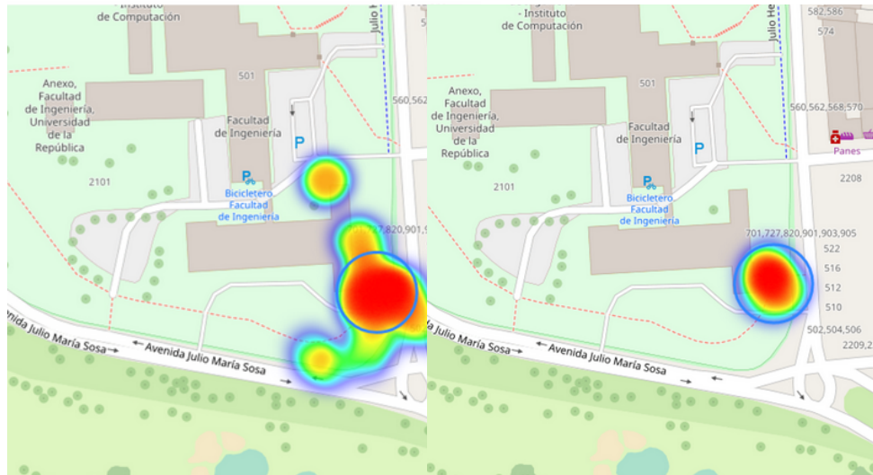
(a) GNSS positions filtered by PDOP < 2 . A low dilution of precision reflects favorable satellite geometry, resulting in more consistent position estimates.
