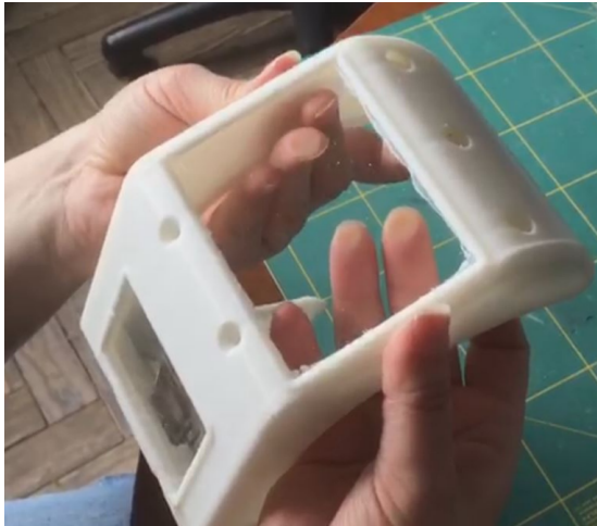
Figure C.1: Acrylic panels placement in the top cover to protect the solar panels.
