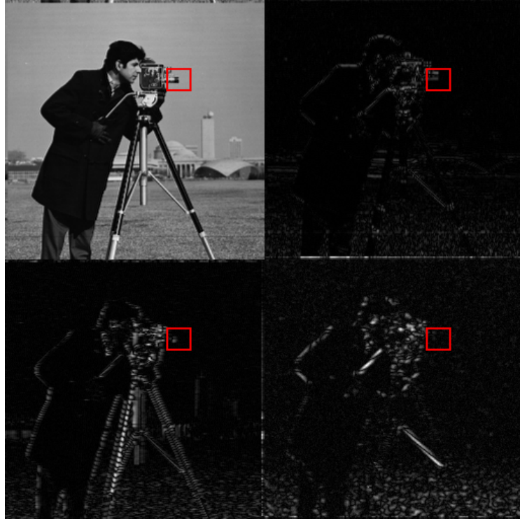
Figure 2.13: Example of a t \times t \times 4 patch in wavelet domain. Note the correlations between coefficients of the summary and the other subbands in corresponding positions.
