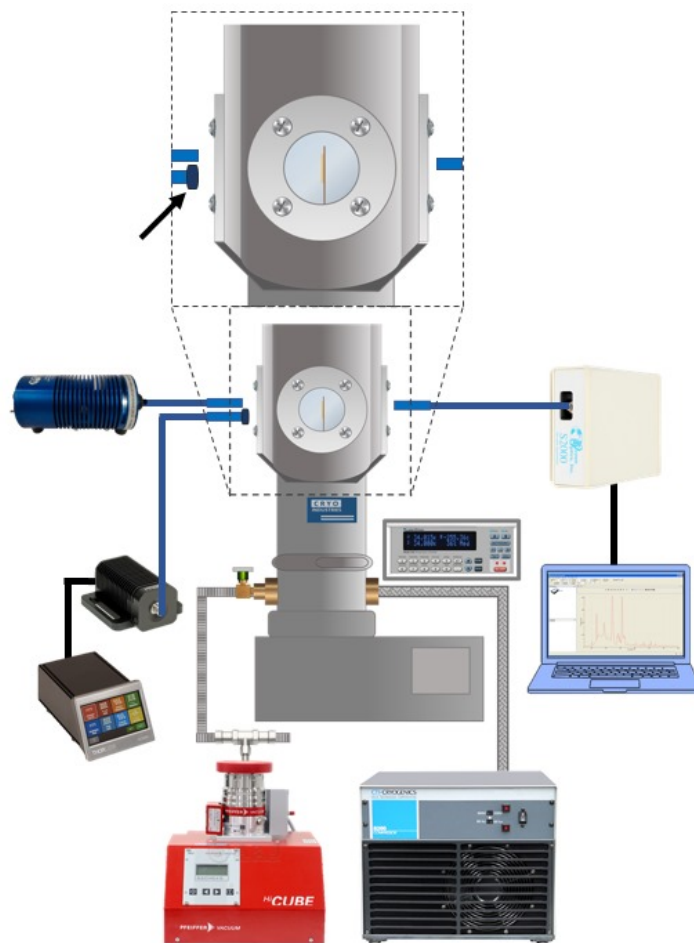
Figure 3.1: Experimental setup used for the low temperature optical measurements. It is showed the cryostat coupled to the HL2000 lamp, the LED and the OOS2000 spectrometer. Figure courtesy of B.Sc. Carina Cabrera.
