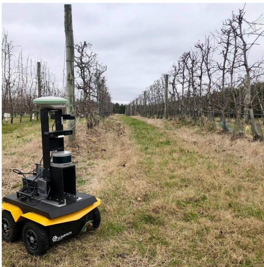
Figure 1. Robot used for detecting and monitoring the quantity and quality of apples
