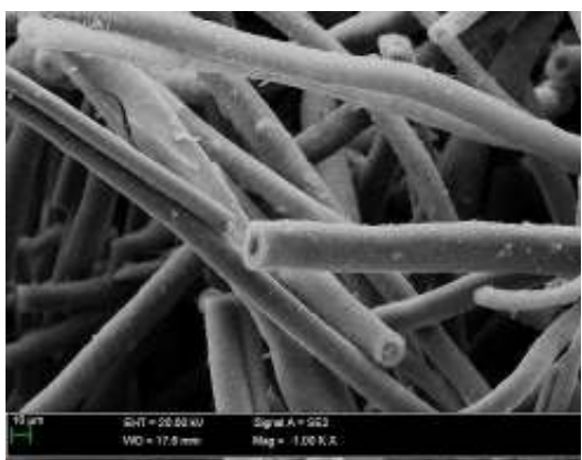
Figure 6.14 SEM image of ACF-KOH, 1000x.
