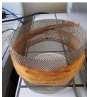
Figure 4.5 Stainless steel hollow cylindrical mesh that was placed inside the muffle.
