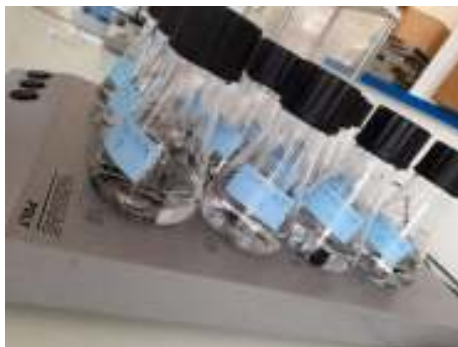
Figure 4.18 Multipoint stirring plate where the experiments were left stirring at room temperature.
