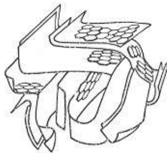
Figure 2.2 Schematic representation of the microstructure of the AC (Bansal et al. 1988).
