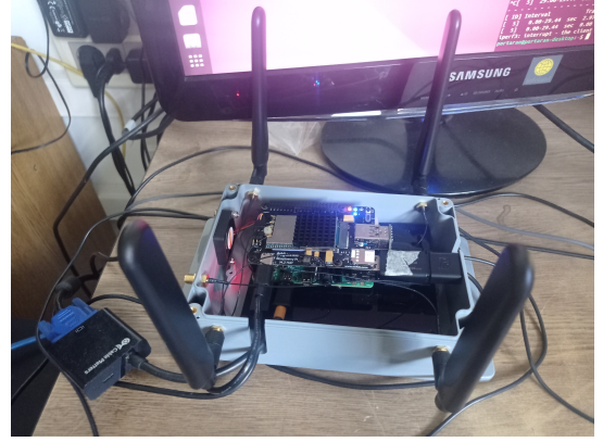
Fig. 1. Sixfab 5G Development Kit installed on Raspberry Pi 4.
