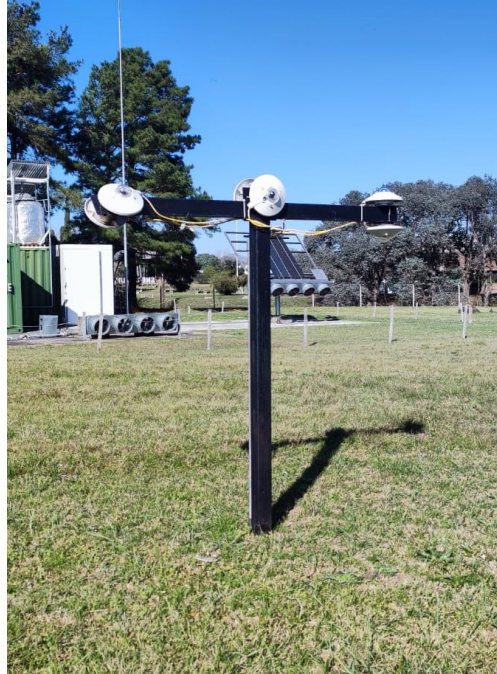
Figure 1: Experimental setup to measure the albedo of the ground surrounding the test bench (both instruments on the right; the others are for inclined solar irradiance, not used in this study).
