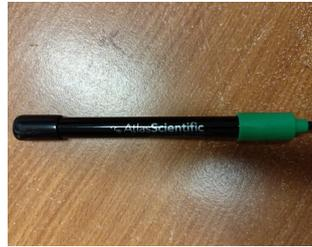
Figura 2.3: Sonda Conductivity Probe K1.0 .
