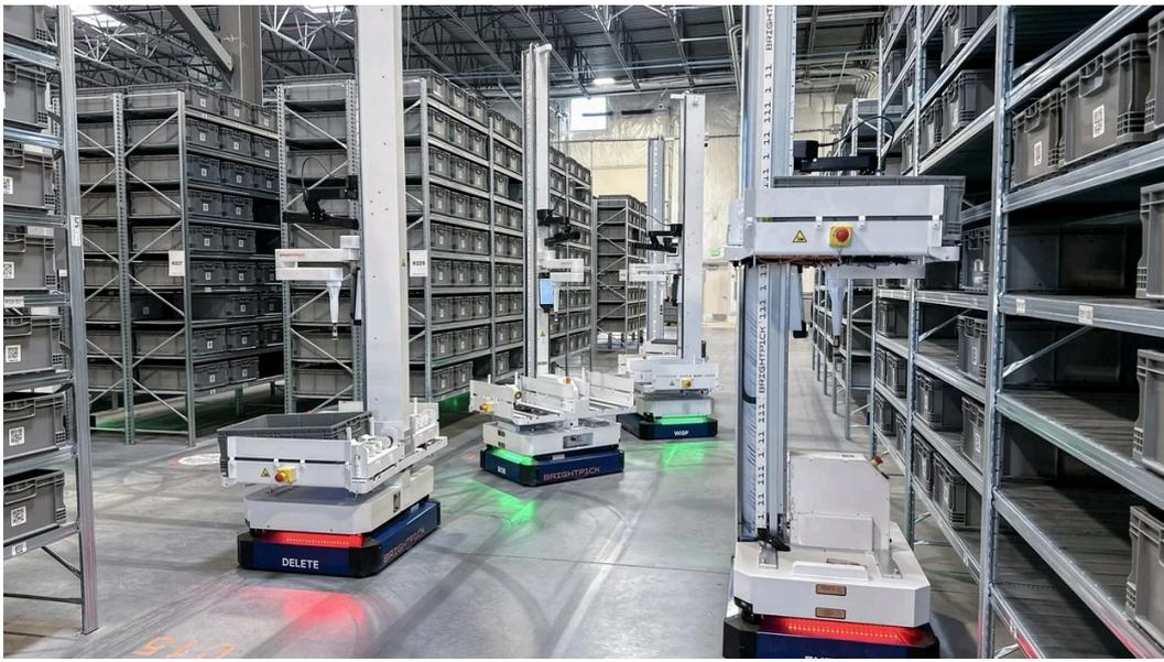
Figura 38: Sistema de AMRs "in-aisle" picking [44].
