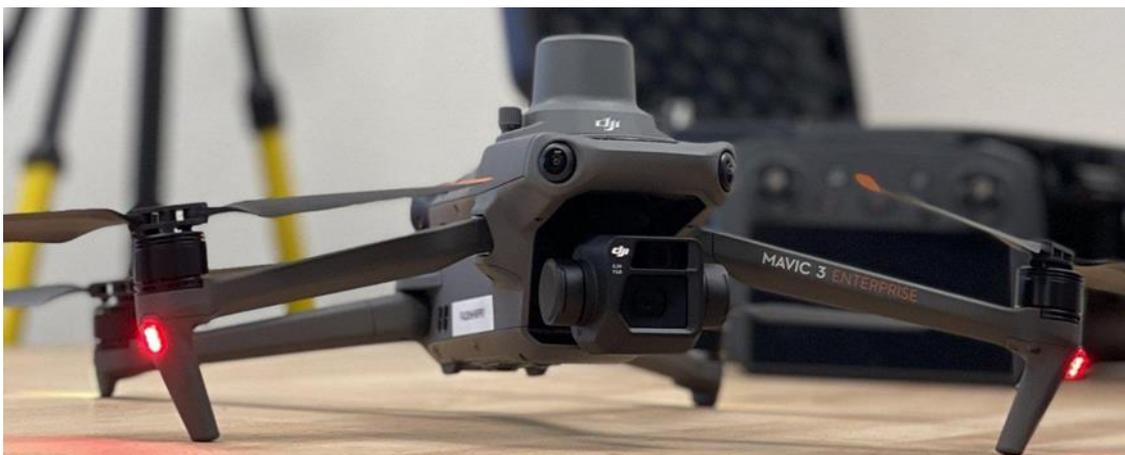
Imagen 10: Mavic 3 Enterprise RTK. Fuente: [enterprise.dji.com](https://enterprise.dji.com)
