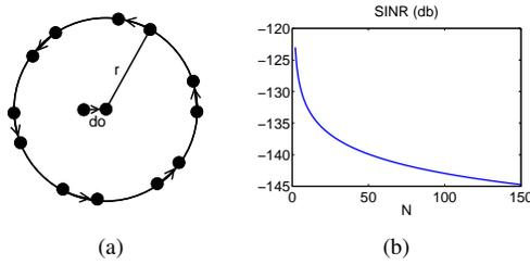
Fig. 1. (a) Example topology and (b) Mean SINR for the receiver located at the center of the circle.
