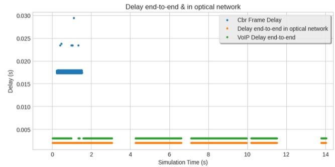
Fig. 4. Graph showing the end-to-end delay and the optical network delay for both traffic profiles: VoIP and CBR.
