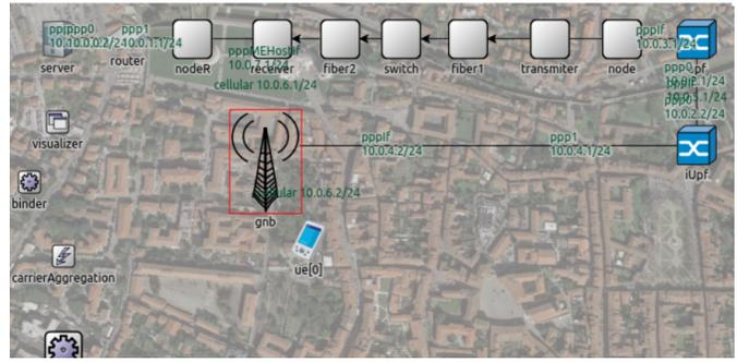
Fig. 3. Example of one-way path topology (OMNeT++ graphical interface). In this topology, one UE is represented.
