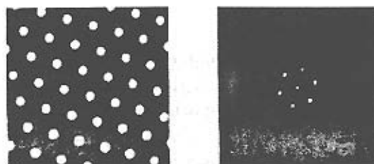
Figure 1.6: Hexagonal pattern produced by the intensity of two counterpropagating beams that have crossed a rubidium cell [146]
