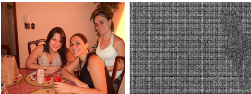
Figure 5.15: A forged image (left) where the woman on the right has been introduced by splicing, and its noiseprint (right). The inconsistencies caused by the manipulation are visible in the extracted noiseprint. Figure obtained from [26].
