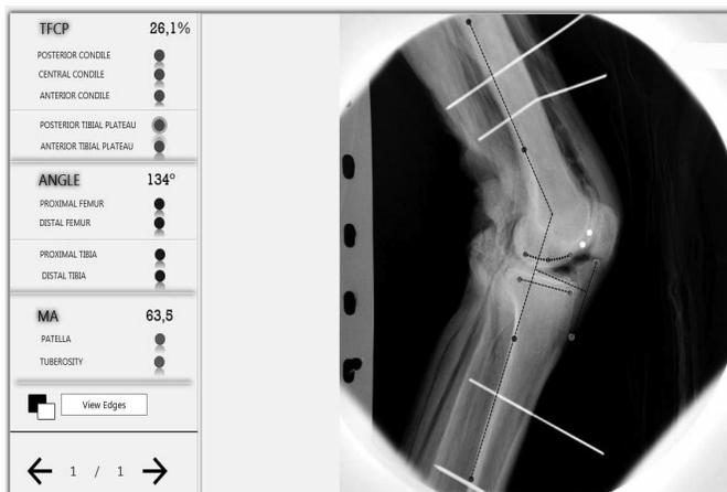
Fig. 3. Screen of CINARTRO software. On the left side the fiducial points are displayed and the operator click on one of them before marking the image on the right. As the points are marked, the software displays in bold characters on the left side of the screen, the angle of the Femoral-Tibial extension and the Moment Arm (MA) once the Tibio Femoral Contact Point is automatically determined and shown on the very image.
