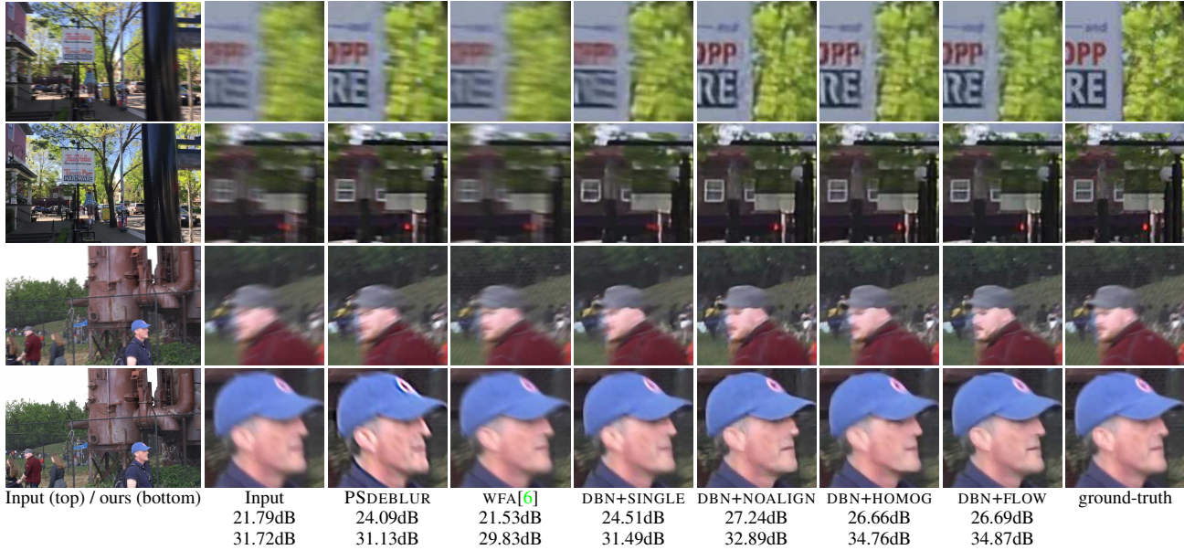
Figure 4: Quantitative results from our test set, with PSNRs relative to the ground truth. Here we compare DBN with a single-image approach, PSDEBLUR, and a start-of-the-art multi-frame video deblurring method, WFA [6]. DBN, achieves comparable results to [6] without alignment, and improved results with alignment.
