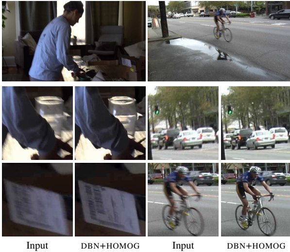
Figure 7: Our proposed method can generalize to types of data not seen in the training set. The first example shows a low-light, noisy video, and the second shows an example with motion blur, rather than camera shake. The biker is in motion, and is blurred in all frames in the stack, but the network can still perform some moderate deblurring.
