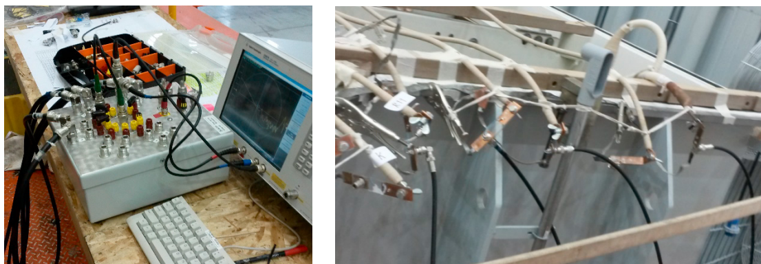
Fig. 5. Connection box and VNA used in admittance measurements (left), and connection to transformer using shielded cables (right).
