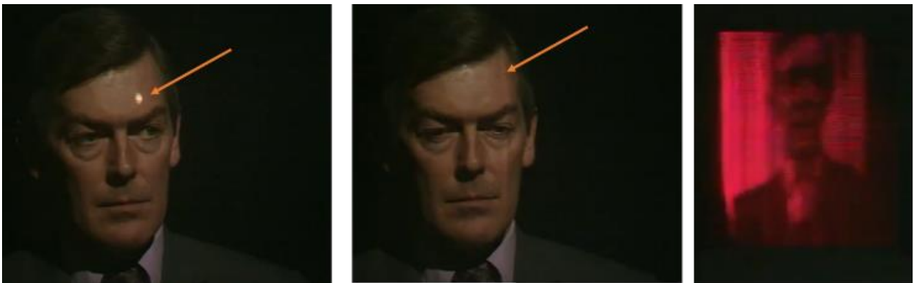
Figure 11. Scanning by Baird's system. On the left, a point of light with the disk fixed. In the center, a vertical sweep line with the disk spinning. On the right, image obtained from the receiver [12].
