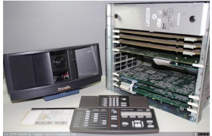
Figure 34. PictureTel System 4000 with Camera, keyboard and CPU Codec [80].
