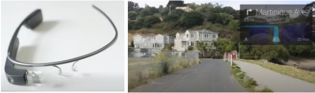
Figure 19 –Google Glass Explorer Edition. Left: Device detail. Right: User's view for navigation directions [41].
