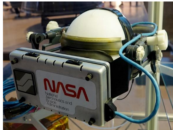
Figure 6 – VR headset prototype, developed in 1985 by Jim Humphries and Mike McGreevy at NASA's Ames Research Center. The system created a computer-generated image of what a pilot might see during a real flight.
