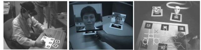
Figure 18 – Video conferencing system with AR, developed in 1999 by Hirokazu Kato. Left: a user in the virtual video conference. Center: AR representation of two users in the video conference. Right: an overlay of the virtual whiteboard shared with the AR elements [34].
