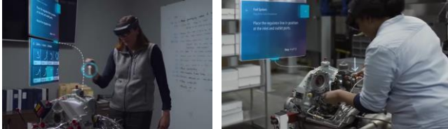
Figure 30 – Microsoft 365 Guides. An operator performs industrial tasks with the support of contextual, 3D work-guides directly superimposed on the physical elements [60].
