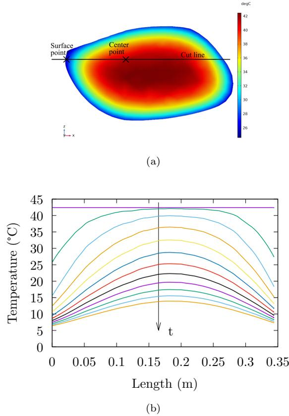
Figure 4: (a) Hind leg section, location of cut line and reference points. Temperature color map at time 2 hours (beginning of cooling process). (b) Temperature profile evolution during slaughter and cooling processes (every 2 hours) along the hind leg cut line.
