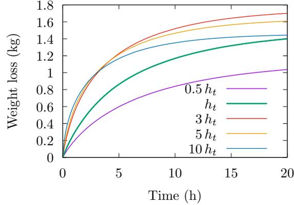
Figure 11: Cumulative weight loss during cooling process for different values of convective heat transfer coefficient.
