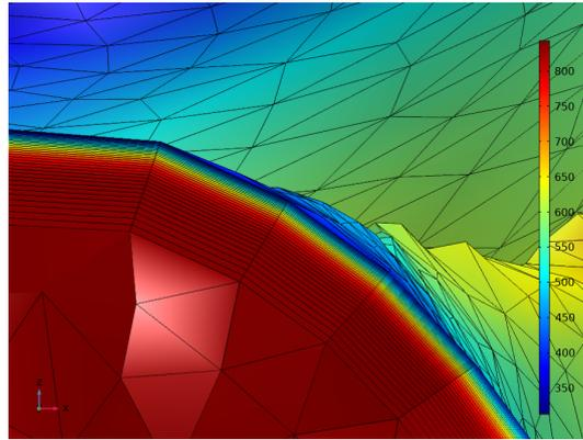
Figure 7: Meat water content distribution in leg section at the end of cooling process (22 hours), overlaid with the boundary layer mesh.
