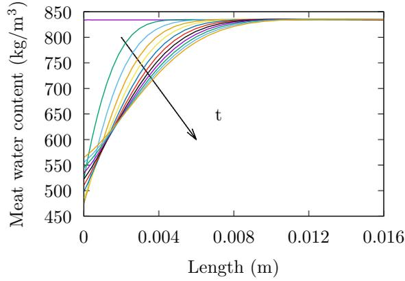
Figure 8: Meat water content profile evolution during slaughter and cooling processes (every 2 hours) along the leg cut line, in a thin layer near the surface.
