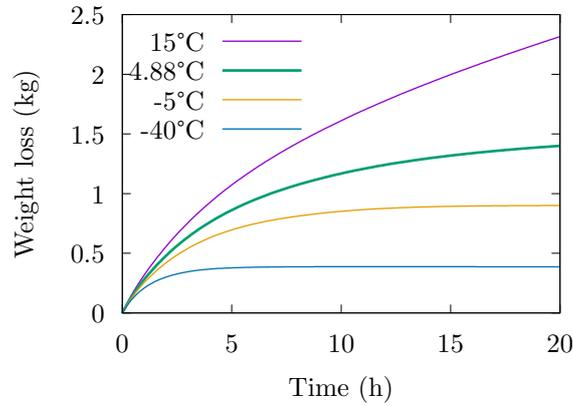
Figure 13: Cumulative weight loss during cooling process in different scenarios of radiative cooling (varying the wall temperature  $T_w$ ), based on reference convective coefficients values.
