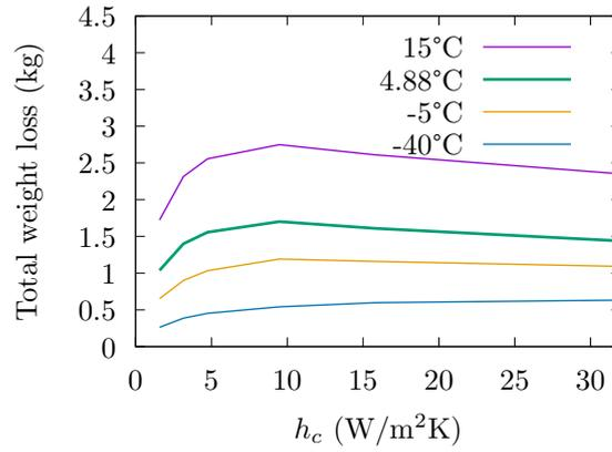
Figure 12: Total weight loss after 20 hours of beef cooling vs convective coefficients. Curves for different radiative heat transfer, varying the wall temperature  $T_w$ .
