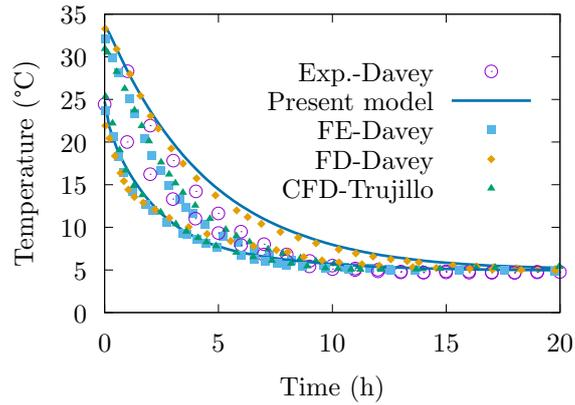
Figure 6: Temperature evolution in surface (down) and center (top) points in loin section during cooling process. Comparison of the proposed model with the experimental values and other models.
