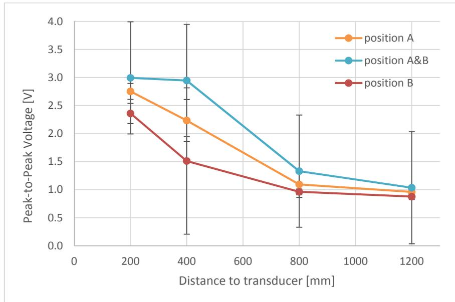
**Figure 4: Sound penetration in water across an industrial size trough using a 600 kHz industrial plate transducer (regions of the twin plate transducer are defined as: A – left region; A&B central region; B – right region).**
