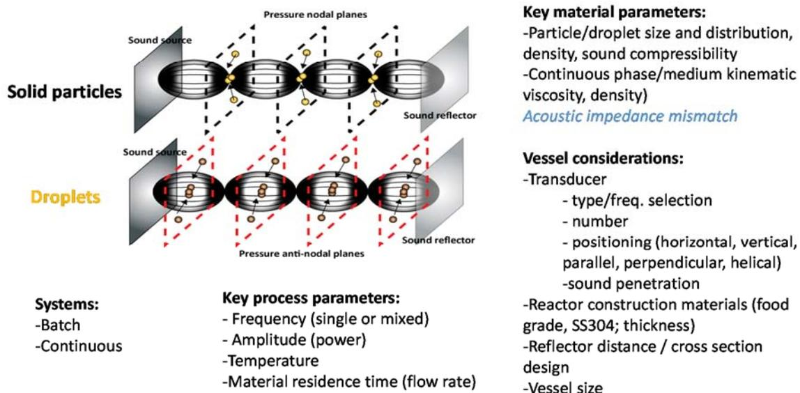
Figure 1: Key design parameters for megasonic reactors
