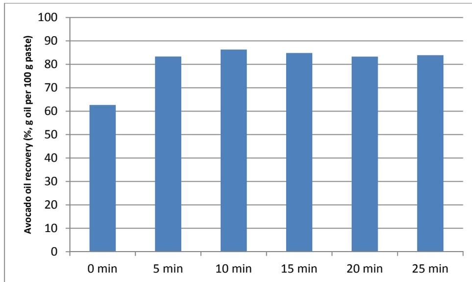
**Figure 7: Oil recovered before and after sonication of avocado water mixture at 1,600 MHz for 5-25 min.**
