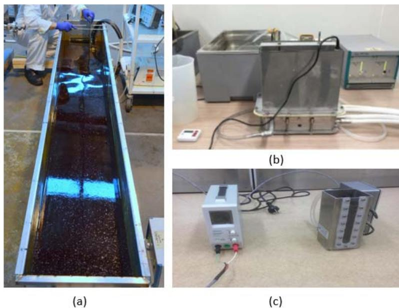
**Figure 3: Megasonic devices for (a) sound penetration studies (2.4 m trough) and (b) palm oil separation studies, (c) avocado oil separation studies**
