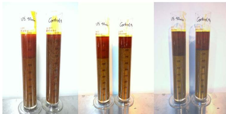
**Figure 6: Decantation cylinders with untreated and megasonic (600 kHz) treated samples at 0 min, 15 min and 3 h at 80°C (left cylinder – sonicated control; right cylinder – non-sonicated control).**
