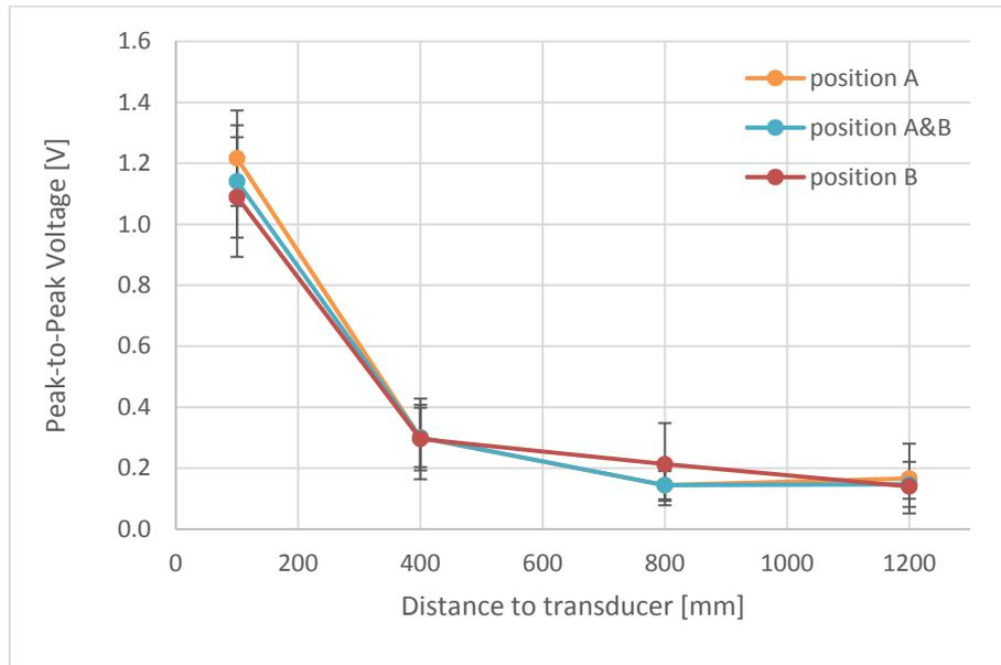
**Figure 5: Sound penetration in an industrial size trough using a 600 kHz industrial plate transducer (regions of the twin plate transducer are defined as: A – left region; A&B central region; B – right region).**
