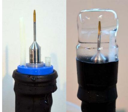
**Figure 2: Hydrophone prototype design including a cooling system and glass barrier for direct measurement in food materials**
