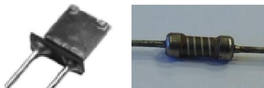
**Figure 1.** Resistors without cover.
