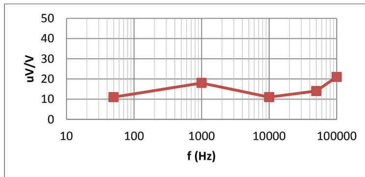
**Figure 5.** AC-DC differences of the prototype in parts in  $10^6$ .
