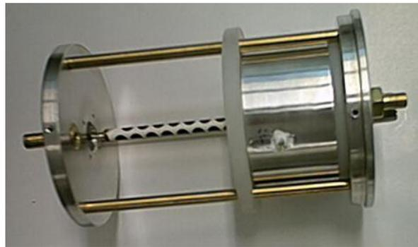
**Figure 2.** Adjustable partial shield to compensate for ground stray capacitances.
