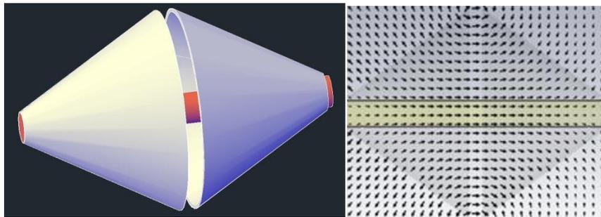
**Figure 3.** Electrostatic shield to null radial electrical fields. Shape and vector field diagrams.
