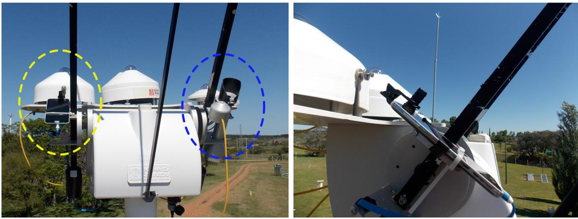
Figure 2: Experimental setup. In the left panel the professional reference equipment (pyrheliometer) and the smartphone can be appreciated. The right panel offers a different perspective of the smartphone alignment.
