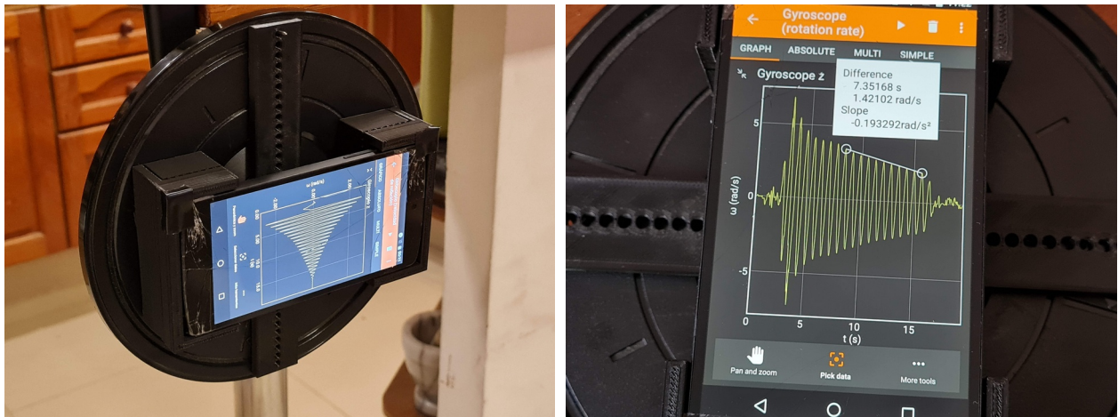
Figure 4. To directly measure the inertia moment the device was hung from a point at its periphery, let it oscillate, and the period of oscillation was registered using the phyphox app (left picture). The period was obtained by the time difference tool over 10 oscillations (right picture).
