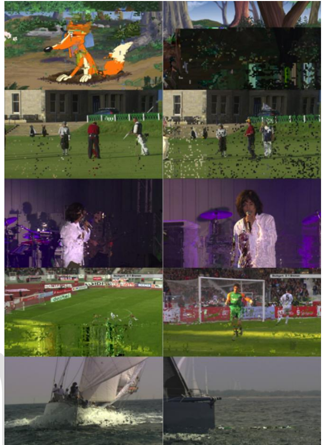
Fig.1 Preview of representative frames showing how transmission errors affect the selected source video clips.
