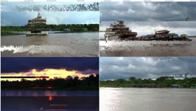
Fig. 4 Preview of representative frames showing how transmission errors affect the frames of recorded video clips from free-to-air DTT.
