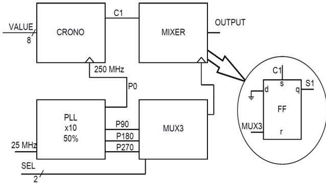
Fig. 1. Simplified diagram of the PLL-based DPWM architecture.
