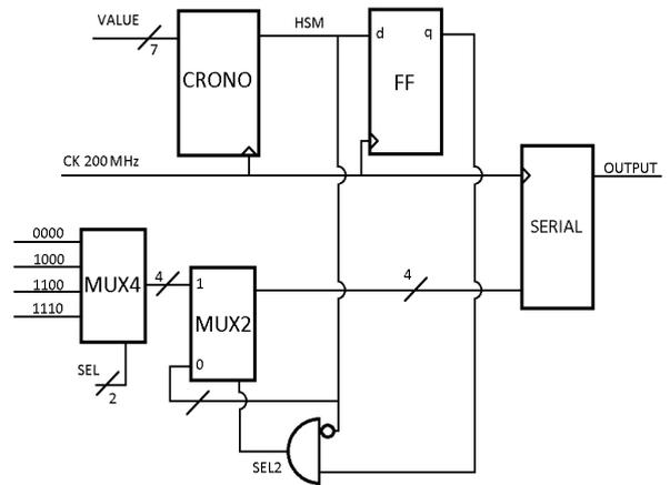
Fig. 2. Simplified diagram of SERDES-based DPWM.
