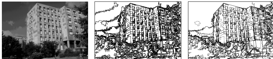
FIG 5. Effect of the maximality condition over the meaningful boundaries of an image. On the left, original image; on the center, DMM-MCB (8987 lines found); on the right, maximal DMM-MCB (517 lines found).
