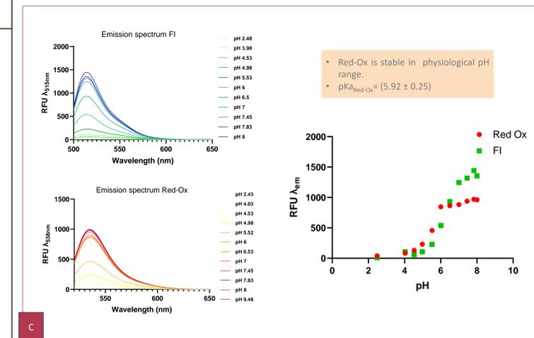
Figure 5. Synthesis and characterization of Red-B and Red-Ox. A) Red-B synthetic route involves 5 steps. Red-Ox was obtained in 3 steps. B) Spectroscopic characterization of Red-Ox, showing its emission and excitation spectra and their differences with its protonated form (Red-Ox)<sup>+</sup>. C) Fluorescence dependence on pH for Fluorescein (FI) and Red-Ox.
