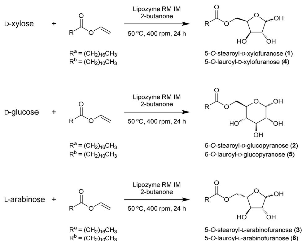
**Scheme 1.** Lipase-catalyzed synthesis of sugar fatty acid esters (1–6), using D-glucose, L-arabinose, D-xylose and fatty acid vinyl esters as substrates.
