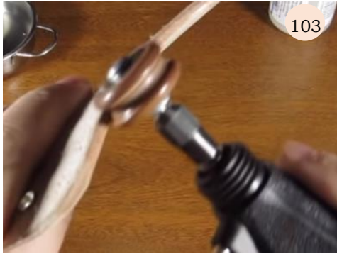
Fifura #103. How to burnish leather the faster and easier way.
