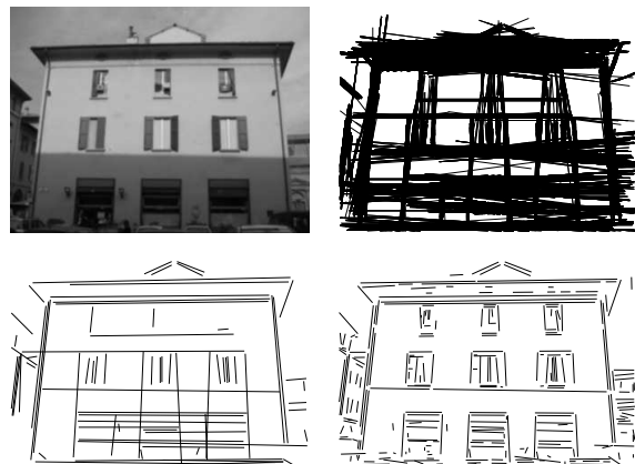
Fig. 1. Up-Left: A digital image. Up-Right: All DMM 1-meaningful segments. Clearly there are many more printed segments than we would be able to perceive, but all of them we do perceive are among these detected segments. Bottom-Left: DMM 1-meaningful segments after exclusion principle. Bottom-Right: Multisegment detections
