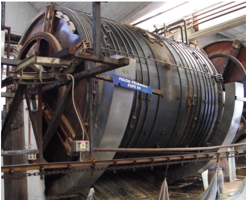
Fig. 1. Tannery barrel hosting the sensor
