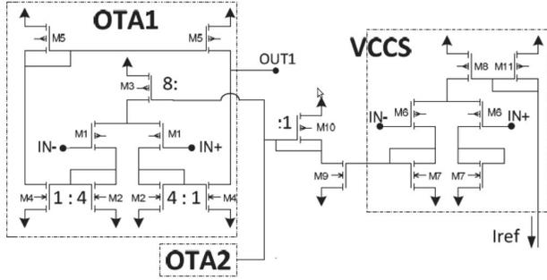
Figure 4. Schematic of the OTA(Transconductor) and VCCS.
