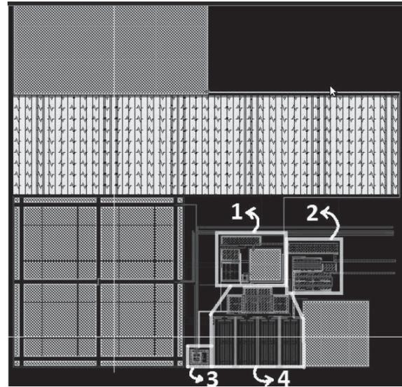
Figure 5. Layout view of the filter with Automatic Tuning.
