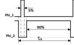
Figure 2. Phases of the switched capacitor
