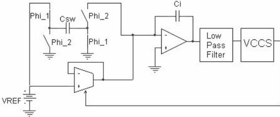
(b) Direct implementation of the tuning scheme of (a) for Gm-C filters
