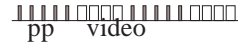
Figure 2: Probe packets (pp) and probe video (video) are sent together in order to map the state of the network into the QoS metric measured over the video sequence.
