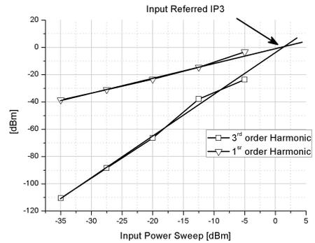
Figure 11:  $IIP3$  of the differential circuit
