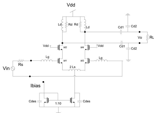
Figure 1: Differential CS-LNA designed. [7](Input biasing and matching not shown)
