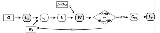
Figure 4: CS-LNA design methodology using ACM model
