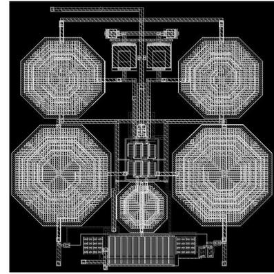
Figure 5: Final layout of the CS-LNA under fabrication.
