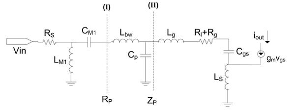
Figure 2: CS-LNA small signal model, with input adaptive network  $C_{M1}$ / $L_{M1}$ , bonding inductance  $L_{bw}$  and pad capacitance  $C_p$  included.
