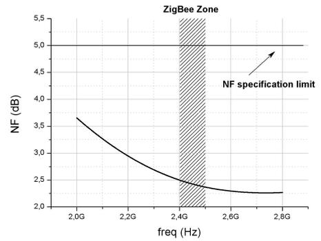
Figure 10:  $NF$  simulation of the differential circuit including bias and package
