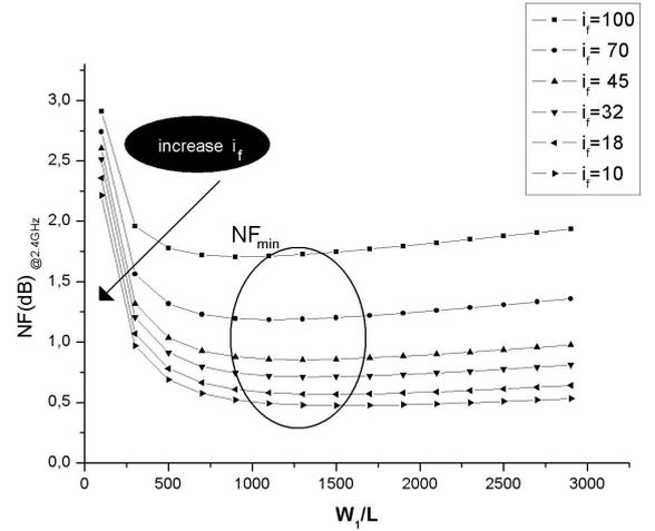
Figure 3:  $NF$  versus  $W/L$  ratio for various  $I_f$  values obtained with ACM model.
