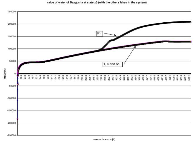
Fig. 2. Value of the water of Baygorria at state  $x_3$  - with the other lakes in the system. (Reversed time axis in hours).
