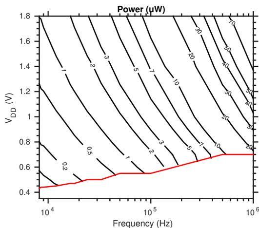
Fig. 5. PTT processor core power consumption vs  $V_{DD}$  and operating frequency.
