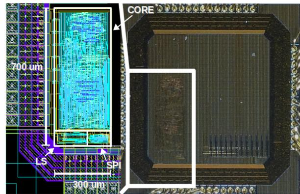
Fig. 4. Fabricated IC microphotograph and PTT processor layout.
