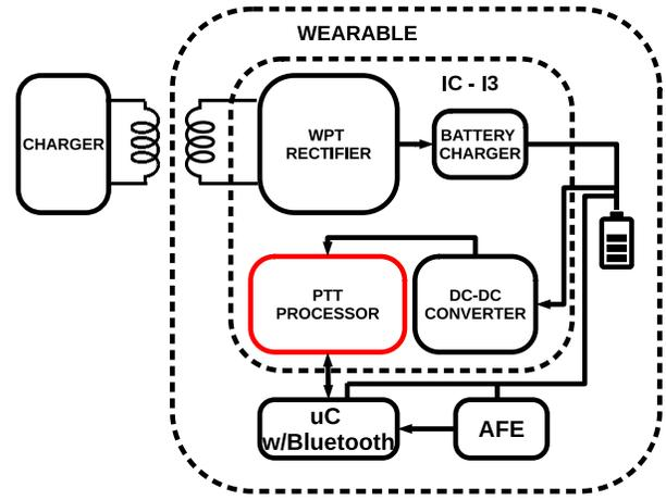
Fig. 2. Wearable device block diagram.
