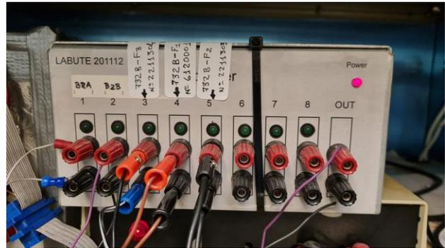
**Fig. 3.** Resistance scanner for temperature measurements.
