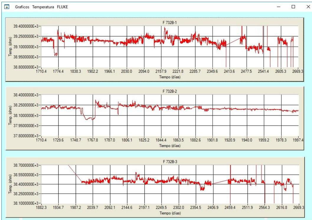
**Fig. 7.** Thermistor resistance values of three Fluke-732B, during 7 years.
