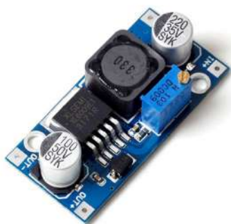
Figura 4.21: Convertor Boost regulable XTW-SY-8
