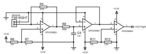
Fig. 3. Signal Conditioning Circuit (right channel).
