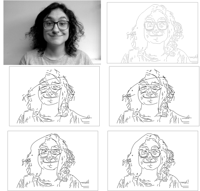
Fig. 6. From left to right, downwards: original image; detected edges; feasible curves without enhancements; feasible curves after splitting the original curves with curvature threshold of 120 degrees; feasible curves after splitting the original curves with curvature threshold of 150 degrees; feasible curves after splitting the original curves with curvature threshold of 120 degrees and a maximum length of 50 pixels per curve.
