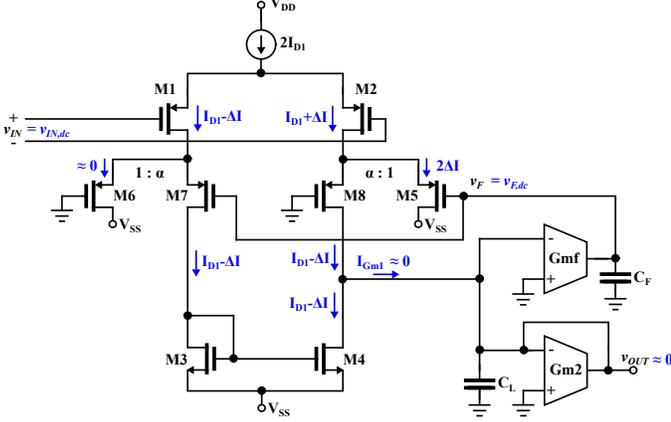
Fig. 7. Block diagram of the proposed architecture. The steady state condition of the dc input blocking mechanism is highlighted, this implies that the current through M8 equals the one by M7 and  $I_{Gm1} \approx 0$ .
