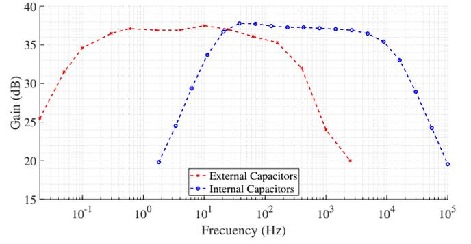
Fig. 21. Pre-amplifier frequency response for chip 6. The bandwidth can be programmed between 0.1 Hz and 11 kHz.
