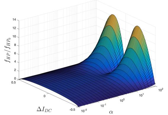
Fig. 11. Variation of normalized  $f_{HP}$  as a function of  $\alpha$  and  $\Delta I_{DC}$
