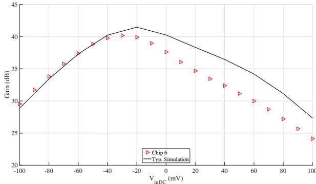
Fig. 20. Variations of the gain with a dc input voltage ( $V_{inDC}$ ) for Chip 6.
