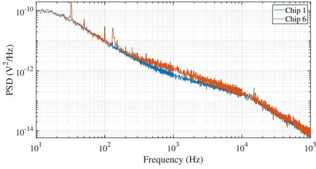
Fig. 15. Input-referred noise power spectral density
