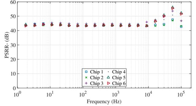
Fig. 18. PSRR- measured for the six chips.
