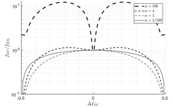
Fig. 12. Cross section of Fig. 11. Variation of normalized  $f_{HP}$  as a function of  $\Delta I_{DC}$  for  $\alpha = \{0.01, 1, 4, 100\}$
