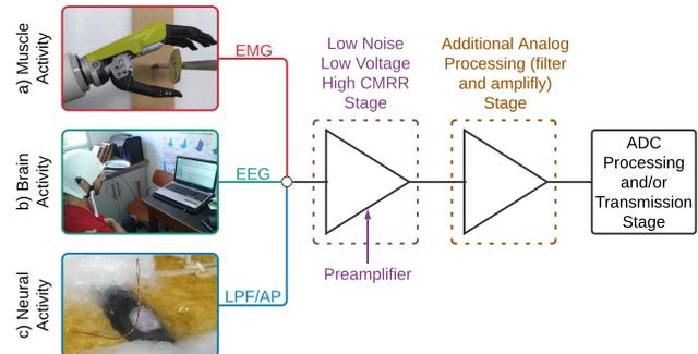
Fig. 1. Typical use of a preamplifier as the input stage of a biopotential recording device: a) Osseointegrated neural prosthesis [3], b) Wireless EEG System [4], and c) Weakly electric fish recording [5].
