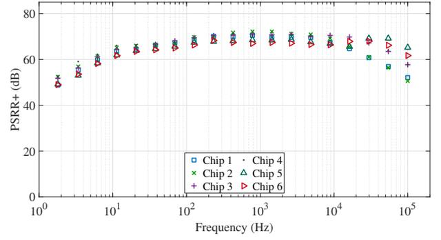
Fig. 17. PSRR+ measured for the six chips.
