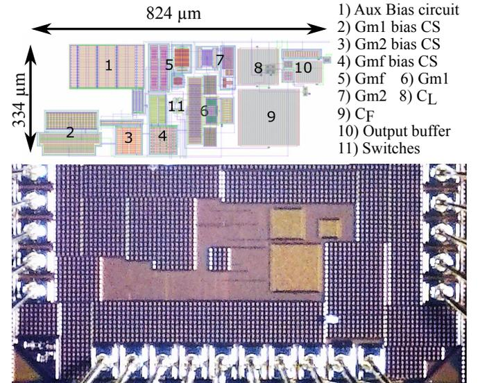
Fig. 13. Overview of the preamplifiers layout (above) with a microphotograph of the manufactured chip (below). CS stands for “Current Source”.
