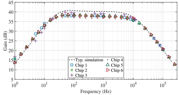
Fig. 14. Preamplifier frequency response.
