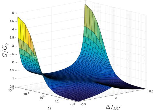
Fig. 9. Variation of the normalized gain  $G$  as a function of  $\alpha$  and  $\Delta I_{DC}$
