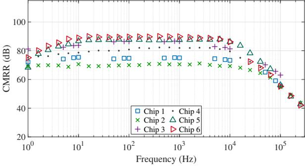
Fig. 16. CMRR measured for the six chips.
