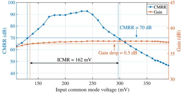
Fig. 19. Chip 6 measurement of input common-mode range (ICMR). Gain (orange) and CMRR (blue) measurements for different dc input common-mode voltages (referred to ground).
