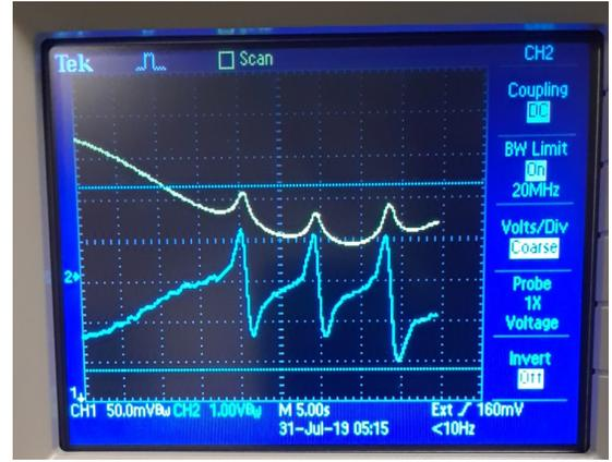
Fig. 10. Frequency spectrum from the reported setup (lower blue trace) and a reference spectrum (upper yellow trace) shown directly in an oscilloscope.
