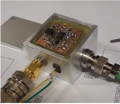
Fig. 8. Miniaturized saturated absorption spectrometer (open view).
