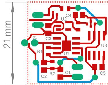
Fig. 4. PCB layout (top view): top layer in red, bottom layer in blue, pads and vias in green.
