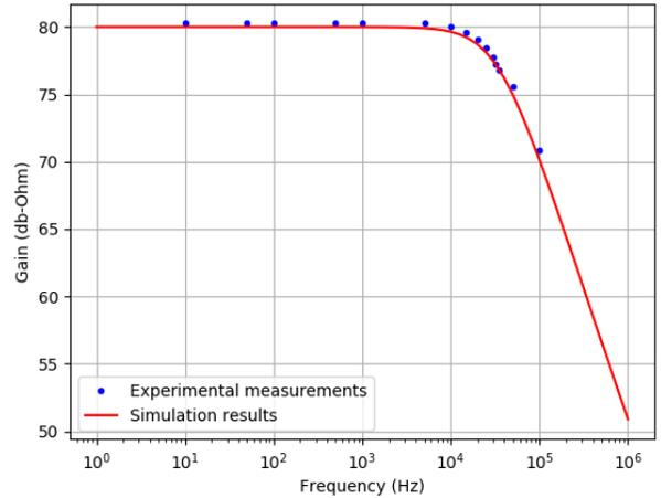
Fig. 7. Frequency response of the amplifier.
