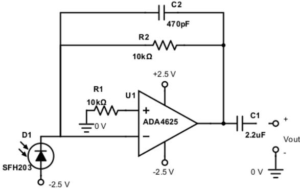
Fig. 2. Amplifier schematic.
