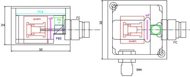
Fig. 5. Case mechanical design: top view (right) and side view (left). Different components are marked in colour: fiber coupler (FC) in black, polarized beam-splitter (PBS) in blue, quarter-wave-plate (WP) in pink, photo-diode (PD) in green, PCB in light-blue, SMA connector in black, and the heater in red.
