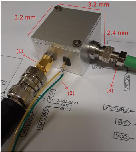
Fig. 9. Miniaturized saturated absorption spectrometer (closed view). The output to the oscilloscope (1), the power supply connector (2), and the input laser source (3) are highlighted in the figure.
