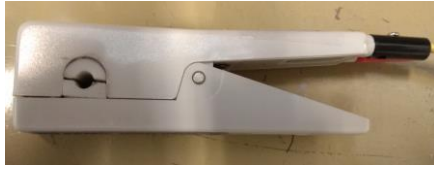
Fig. 4. Clamp-on transformer used in this project, with isolated supplements to centre the cable in its hole.
