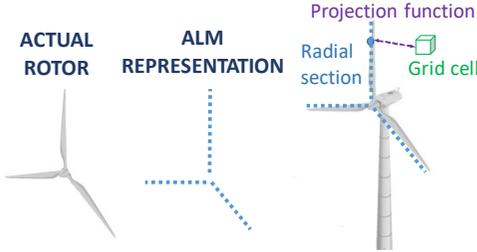
The main cause for the overprediction of aerodynamic loads near the tip are related to a missing induction generated by the formation of a viscous vortex core, originated from the 3D smearing of the forces [2].
