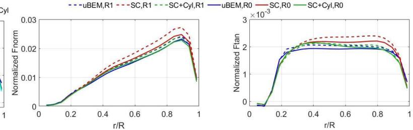
Figure 3. Mean normalized loads along the blades (left: normal force, right: tangential force)..
