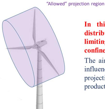
**In this work the aerodynamic forces are distributed using a 3D Gaussian function, limiting the projection region to a cylinder confined within the rotor disk.**
