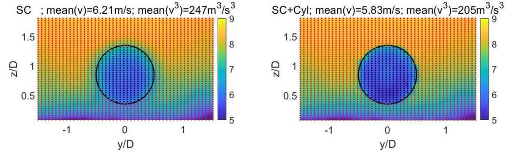
Figure 2. Mean streamwise velocity component at a vertical plane passing through the rotor plane. Black and red dots: points with interpolated data from the CFD grid outside and inside the rotor disk, respectively. The title of each subplot includes the mean streamwise velocity component and the mean value of the kinetic energy flux per unit mass. Smearing factor: E1.
