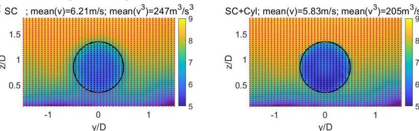
Figure 2. Mean streamwise velocity component at a vertical plane passing through the rotor plane. Black and red dots: points with interpolated data from the CFD grid outside and inside the rotor disk, respectively. The title of each subplot includes the mean streamwise velocity component and the mean value of the kinetic energy flux per unit mass. Smearing factor: E1.
