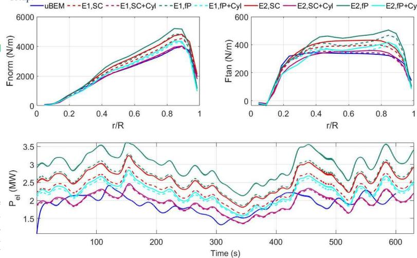
Figure 1. Mean normal and tangential loads along the blades (top, left and right respectively) and electric power time history (bottom). Smearing factor: E1 and E2.
