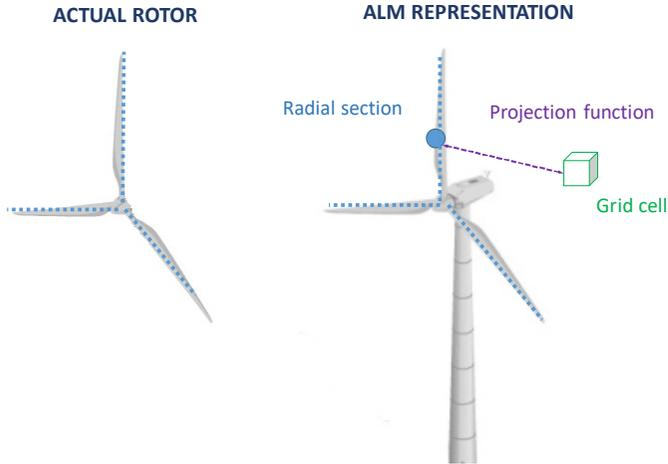
If the aerodynamic forces are projected onto the numerical domain outside the rotor disk, a reduced force field is applied to the fluid particles that may pass through the rotor. As a consequence, the velocity at the lines representing the blades is larger and the wind turbine will capture more power. This is particularly worst when using coarse spatial resolutions.
