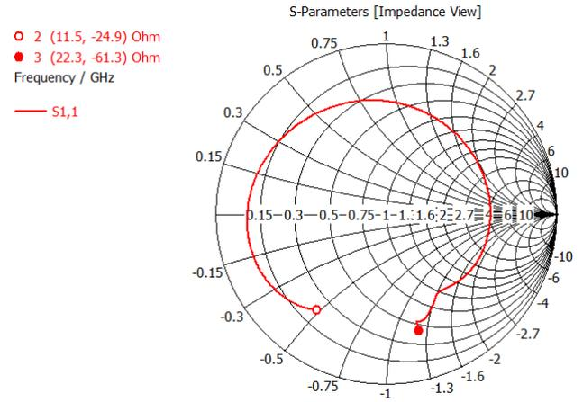
Fig. 3. Simulation of the  $S_{11}$  parameter using the SPIDA antenna model.
