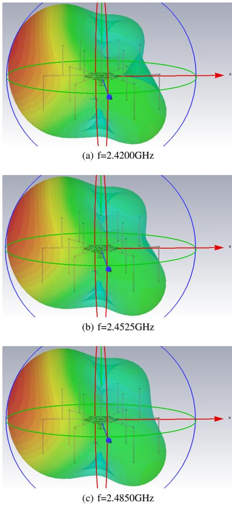
Fig. 4. Simulated Radiation Pattern for the SPIDA antenna model.
