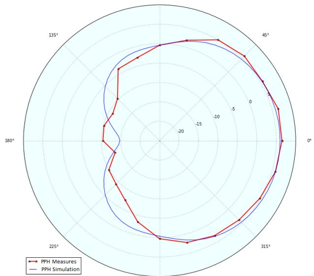
Fig. 7. Measured and simulated gain in H plane for the SPIDA antenna fabricated.
