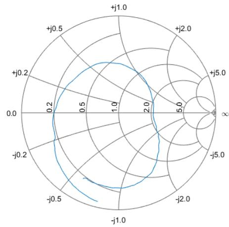
Fig. 6. Measured  $S_{11}$  parameter for the SPIDA antenna fabricated.
