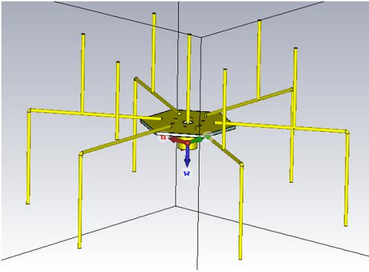
Fig. 2. SPIDA antenna model used in the simulator.
